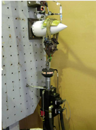
Figure 9: Radome Hydraulic Pull Setup [10]
